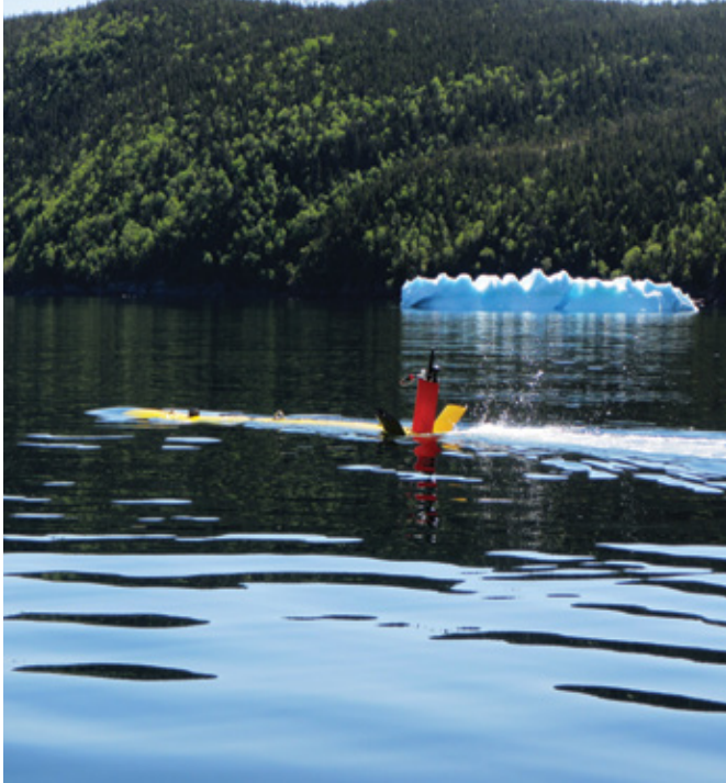
The AUV was used to map the sea floor of Smith Sound for the REALM project.
