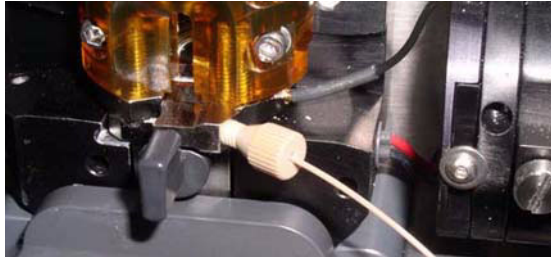
Figure 6-1 Closed-loop nozzle installed in flow cell
