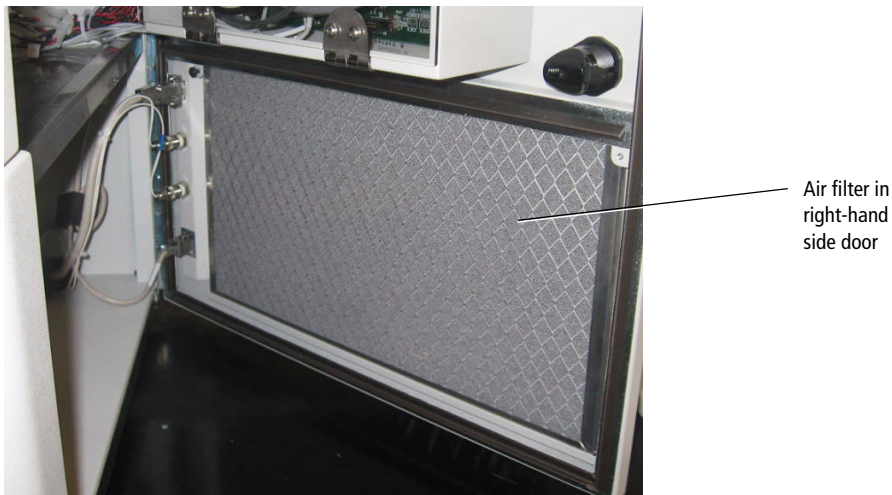
Figure 6-18 Changing the air filter
