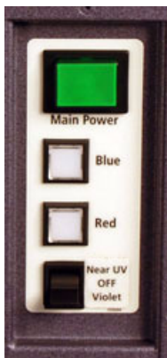
Figure B-2 Violet/Near UV laser toggle switch
