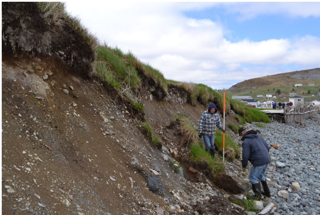
Figure 1: Shoreline erosion along the eastern perimeter of the site.
